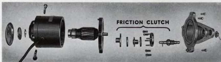
Fig. 74 EXPLODED VIEW OF FOLLOW-UP MOTOR
