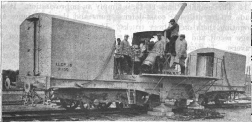
OUTRIGGERS AND WORKING PLATFORMS IN POSITION FOR ACTION.
