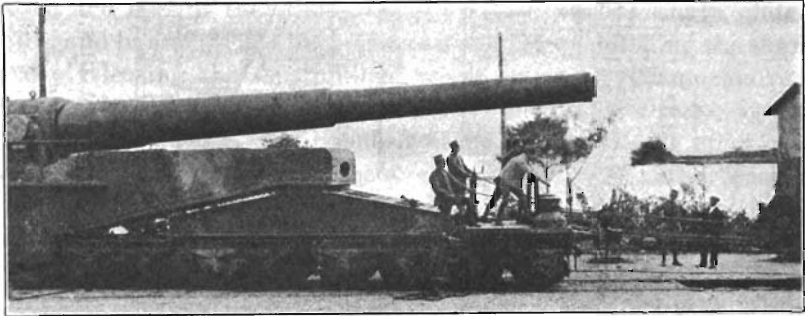
TRANSLATING MOUNT WITH HAND WINCH AND CABLE.
